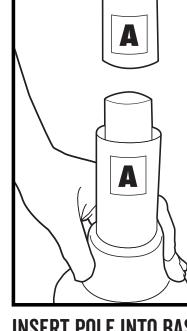
**2.** INSERT POLE INTO BASE, MATCHING "A" TO "A". TWIST TO LOCK.
