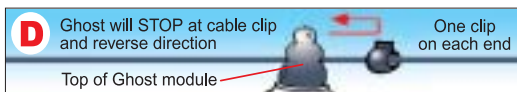
D Ghost will STOP at cable clip and reverse direction. One clip on each end. Position clips along cable to stop ghost where desired.
